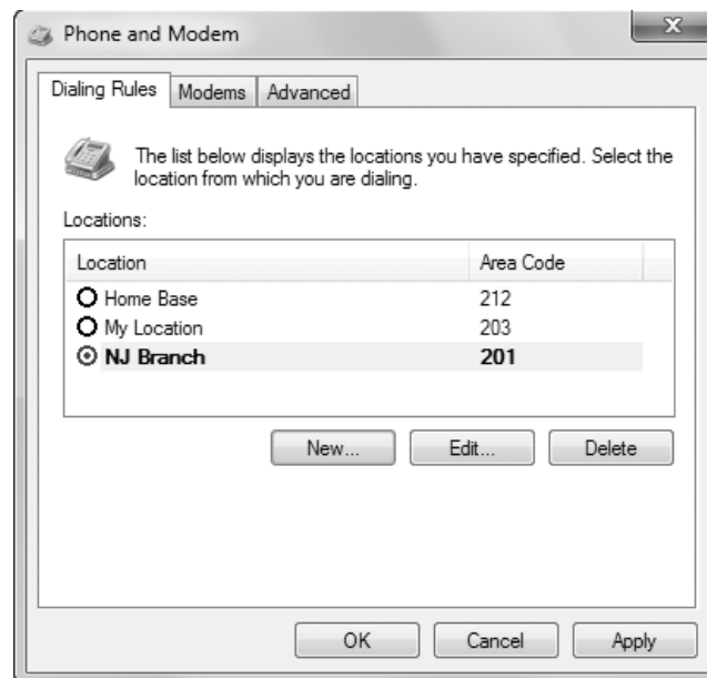
Figure 4: This dialog box has two priorities: to establish rules for dialing out, and to define as many different sets of rules for dialing as you need. If you're setting up dialing properties for a desktop computer, you won't need to change these settings after the first successful call.
